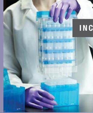
While grasping lower portion of the blister sleeve, lift sleeve up off rack and transfer entire sleeve to an empty rack. Make sure to align sleeve knockouts with latch and rear lid posts.
