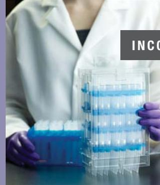
Push down with even pressure on the middle of the top insert, which will slide bottom insert into empty tray.
